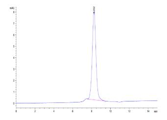
The purity of Human CD160 is greater than 95% as determined by SEC-HPLC.
